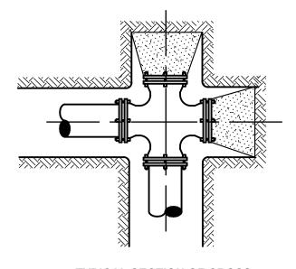
**TYPICAL SECTION OF CROSS** AND 2 PLUG BLOCKING (WHEN DIRECTED BY ENGINEER)
