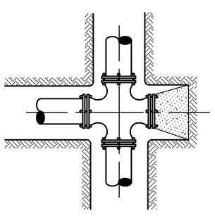
**TYPICAL SECTION OF** CROSS AND BLOCKING (WHEN DIRECTED BY ENGINEER)
