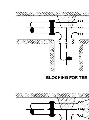
**SPECIAL BLOCKING FOR TEE WITH PLUG** (WHEN DIRECTED BY ENGINEER)
