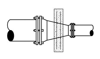
THRUST SUPPORT FOR REDUCER CONNECTION (SIZE TO BE DETERMINED BY ENGINEER)
